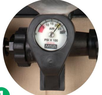
Check that cylinder is fully pressurized. Ensure that the Audi-larm coupling nut is hand tight.
