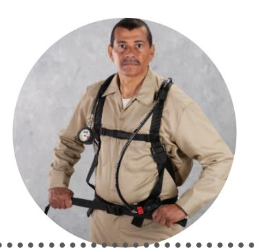
Attach **chest strap** (if used). Fasten waist strap and pull it tight for a snug fit.
