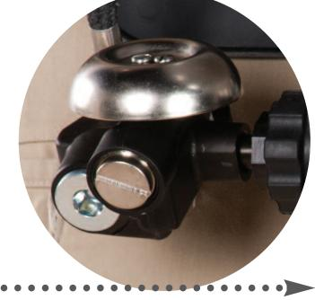
Reach behind and **open cylinder valve** fully. Listen for the alarm to sound briefly. As the pressure rises, the alarm sounds automatically, indicating the alarm is functional.
