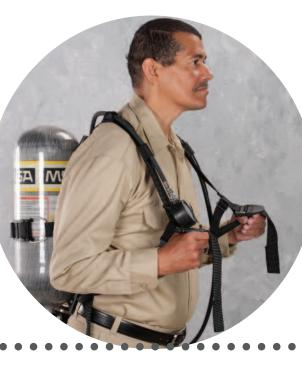
To remove the facepiece, fully loosen the harness straps and pull the facepiece up and away from your face. To remove the carrier harness, press the **belt buckle** release buttons IN. Disconnect chest strap (if used). To loosen the shoulder straps, grasp the release tabs. Push them out and away from your body. Slip your right arm out of the shoulder strap first, then remove the harness.
