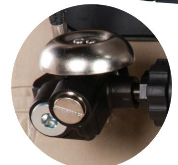
Crack bypass valve slowly to bleed off pressure until gauge needle drops below: 550 psig for 2216 Air Masks or 1125 psig for 4500 Air Masks. The alarm will sound. The alarm must continue to sound until pressure is less than 200 psig. Close bypass fully.
