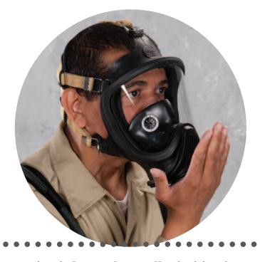
To check **facepiece fit**, hold palm of your hand over inlet connection and inhale. Hold our breath at least 10 seconds. The facepiece should collapse and stay collapsed against your face. If it does not, readjust facepiece and test again.
