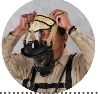
Don facepiece by inserting your chin first. Pull head harness completely over your head and tighten lower (neck) straps.
